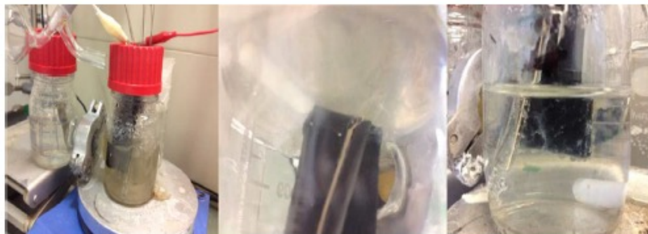
Figure 1. a) Cloudy medium after inoculation of microorganism suspension, b) biofilm formation after 24 h and clarified medium, c) and biofilm after 1 week (multiplying microorganisms) when the medium was exchanged.
